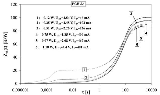
Figure 3: The measured waveforms of transient thermal impedance of the transistor mounted on PCB A1
