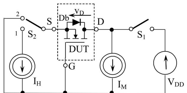
**Figure 1:** The diagram of the measurement set to measure transient thermal impedance of the power MOSFET
