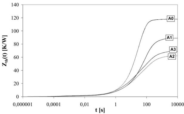
**Figure 4:** The measured waveforms of transient thermal impedance of the transistor mounted on various PCBs
