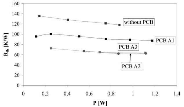
**Figure 5:** The measured dependencies of thermal resistance versus the dissipated power for different mounting methods of the transistor
