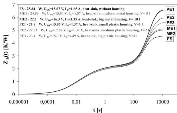
**Figure 6:** The measured waveforms of transient thermal impedance of the transistor mounted on the heat-sink and enclosed in various housings
