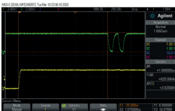
Figure 9: Oscilloscope screenshot of interrupt service routine latency measurement. The yellow trace shows the signal at the digital input, while the green trace represents the signal at the digital output of the microcontroller.
