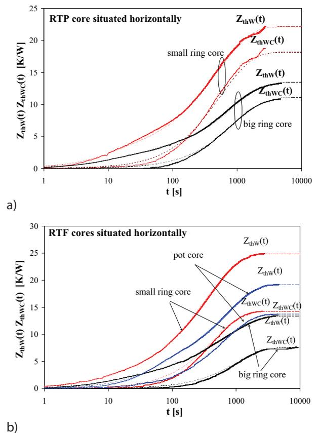
**Figure 6:** Measured (solid lines) and modelled (dashed lines) waveforms of transient thermal impedances in transformers with ring cores RTP (and) and RTF (b) of different dimensions at the stimulation with the direct current of the primary winding and the horizontal orientation of the core
