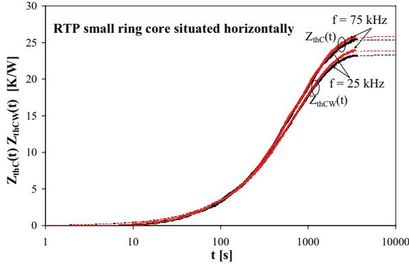
**Figure 11:** Measured (solid lines) and modelled (dashed lines) waveforms of transient thermal impedance of the core and mutual transient thermal impedance between the core and the winding of the transformer with the small ring core RTP at the stimulation with the sinusoidal current of frequency equal to 25kHz and 75kHz
