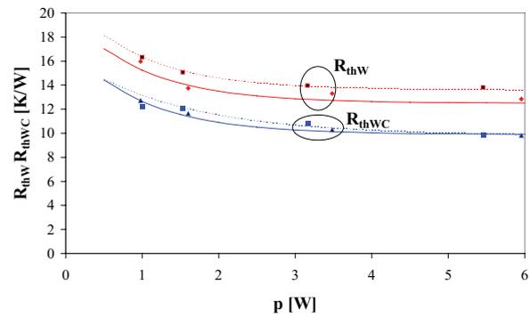
**Figure 12:** Measured (points) and modelled (lines) dependences of thermal resistance of the winding and mutual thermal resistance between the winding and the core on the dissipated power for the transformer with the big ring core RTP at the stimulation with the dc current
