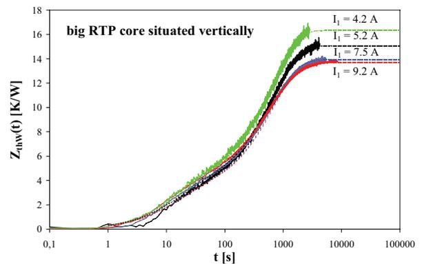
**Figure 13:** Measured (solid lines) and modelled (dashed lines) waveforms of self transient thermal impedance of the winding of the transformer with the big ring core RTP situated vertically at the stimulation with the direct current of different values
