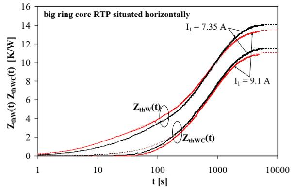
**Figure 9:** Measured (solid lines) and modelled (dashed lines) waveforms of transient thermal impedances of transformers with the large ring core RTP at the stimulation with the direct current of different values
