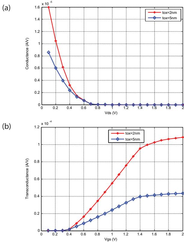
**Figure 9:** Effect of oxide thickness on the (a) conductance at  $V_{gs} = 1\text{ V}$  and (b) trans-conductance at  $V_{ds} = 1\text{ V}$ .
