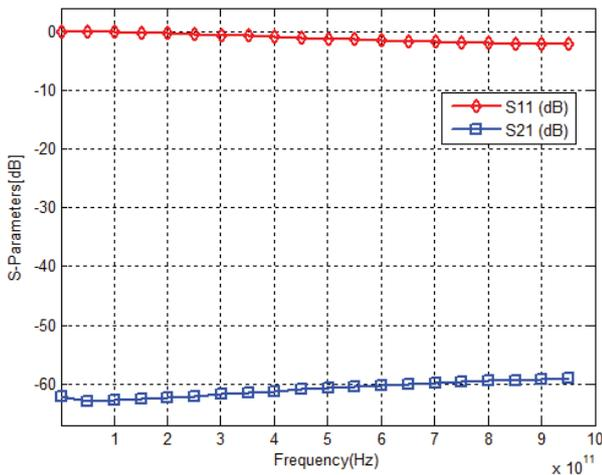
**Figure 11:** S-parameters over a range of high frequencies.
