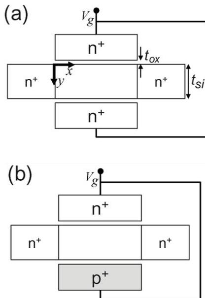
**Figure 2:** (a) Symmetric Double-gate MOSFET, (b) asymmetric Double-gate MOSFET [11].
