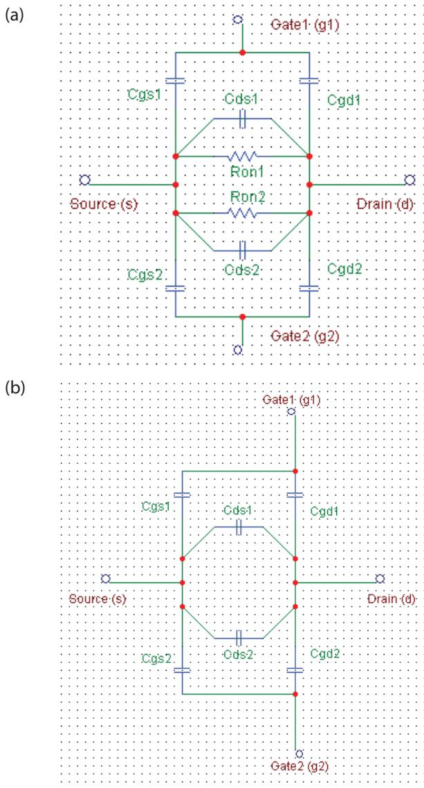
**Figure 4:** Small signal modeling of DG MOSFET at (a) Switch-ON state, and (b) Switch-OFF state.
