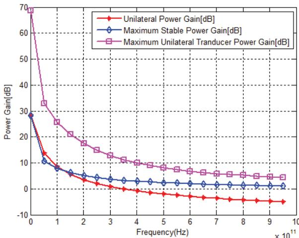
**Figure 12:** Response of the power gain at various frequencies for the DG MOSFET.
