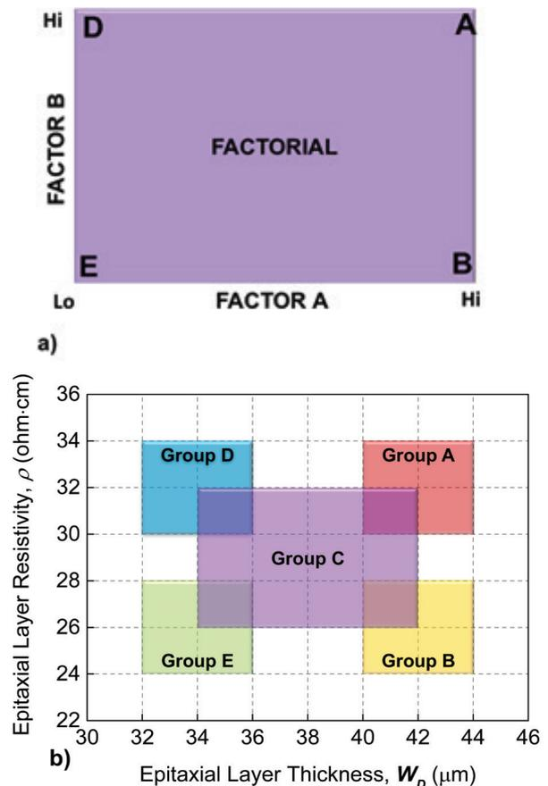
**Figure 5:** a) Two level factorials of DOE, Factor A and B refer to epitaxial layer thickness and epitaxial layer resistivity respectively. b) The location of four corners and centre of the evaluation samples consists of group A, B, C, D and E.
