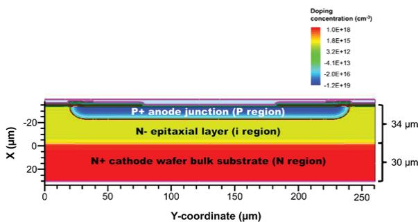
**Figure 3:** P-i-N diode structure with doping profile distribution.
