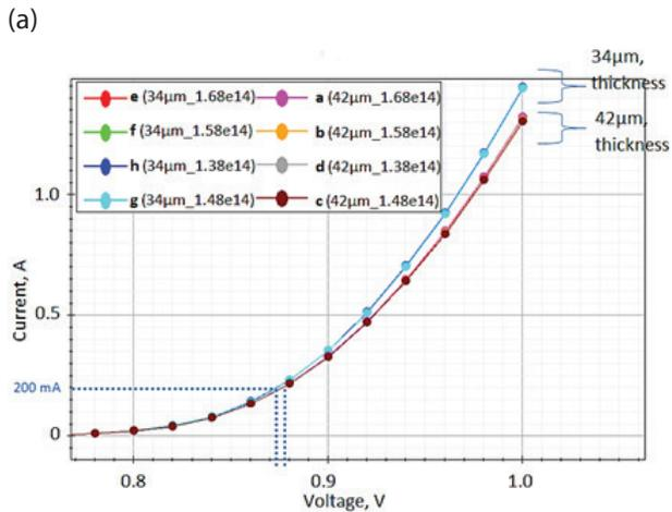
**Figure 6:** I-V characteristics under (a) reverse bias and (b) forward bias for different  $W_D$  and dopant concentrations.
