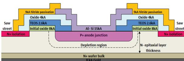
**Figure 2:** Cross-section structure of P-i-N power switching diode.
