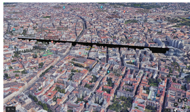
Figure 6: Line-of-Sight estimation using Google Earth in the microwave link design.
