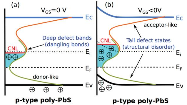
**Figure 4:** Energy band diagram drawn in scale for p-type PbS MOS structure (a) for  $V_G = 0V$  and (b) for  $V_G < 0$  (accumulation regime). Here, only the semiconductor and the interface with the oxide insulator are shown.
