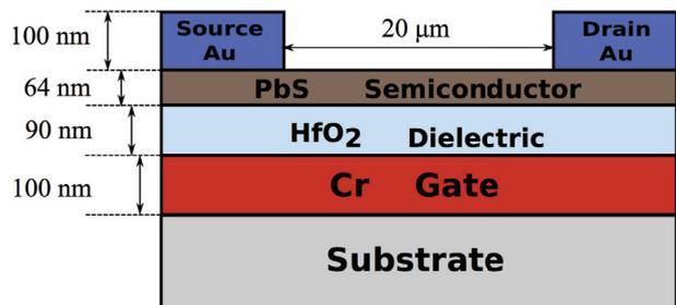
**Figure 1:** Cross section of PbS TFT simulated with  $W=40$  and  $L=20 \mu m$ . We used Cr as gate metal,  $HfO_2$  as dielectric, and Au as source - drain contacts.
