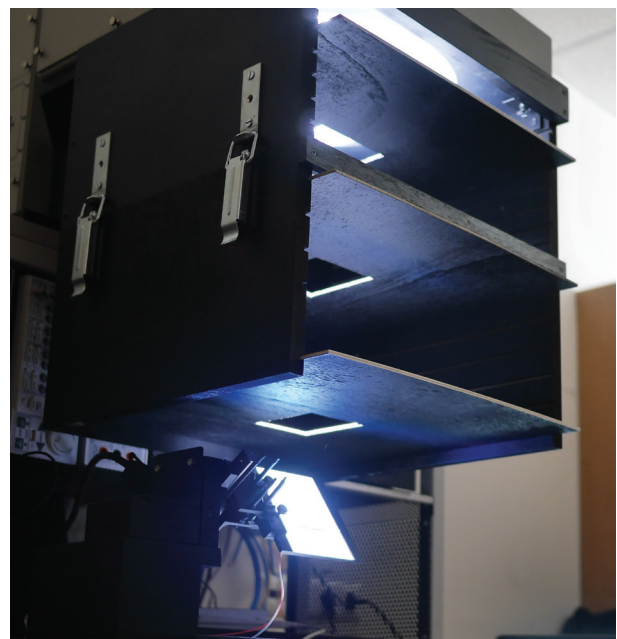
Figure 7: A cascade system of masks that limit the light beam in order to minimize the stray light errors.
